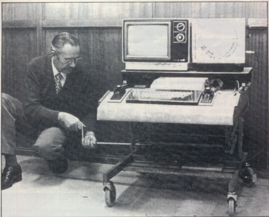
The SCAT (Scanner Apple Touch Keyboard), developed by Centre Industries, the manufacturing division of the NSW Spastic Centre. The SCAT is a self-contained unit incorporating SCAT interface, movable TASA (Touch Activated Switch Array) keyboard and a rotary scanner.
